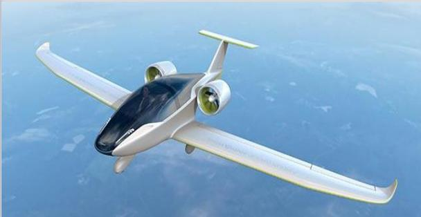
Airbus Group is developing an electric aircraft with Aero Composite Saintonge. The aircraft uses on-board lithium batteries to power the two electric engines.
