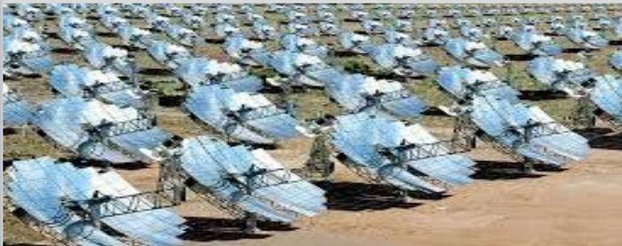
**Solar Thermal** - Uses parabolic disc technology to capture thermal energy based on the solar thermal effect
